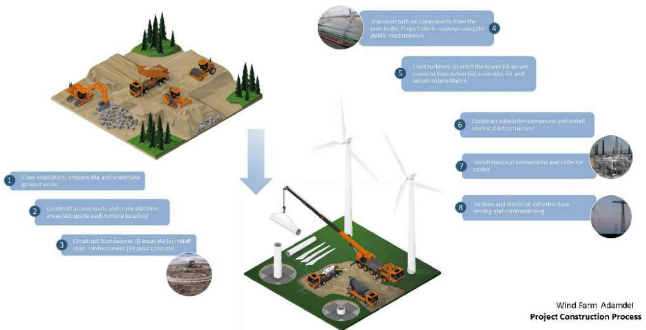
Figure 3-5 Typical wind farm construction process (Source: ERM Draft ESIA)
